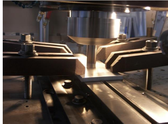
Figure 3: FSW of T-joint in progress.
