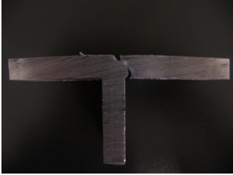
Figure 14: C4 specimen fractured in skin tensile testing.
