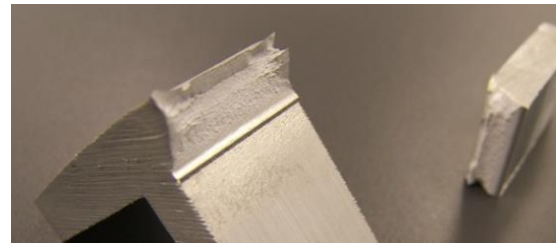
Figure 17: Fracture surface of C5 specimen fractured in skin tensile testing.
